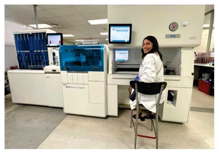
BD Kiestra<sup>™</sup> laboratory automation offer adaptable solutions for sample inoculation, incubation, plate imaging and reading as well as follow-up testing.
